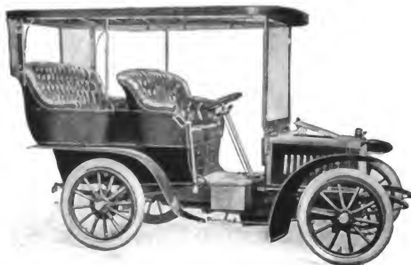
Phaeton Tulip, 1904 Model with Swinging front seat, 4 cylinders, furnished in 15-20 or 30-35 h. p.
